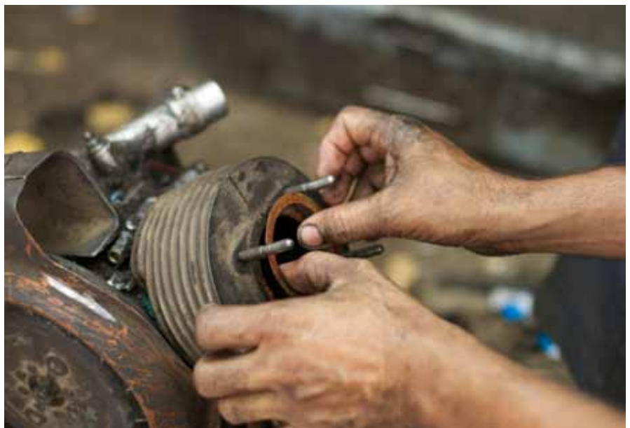
Replacing an asbestos gasket, © ROCA/GAAA
