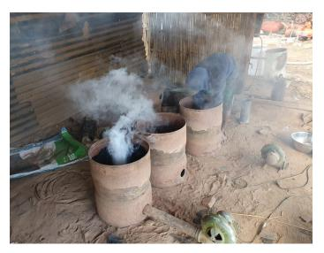
Figure 3. Mercury contaminated cyanidation plant in Indonesia. Tailings stockpiles, liquid releases, emissions from roasted activated carbon laden with gold, mercury and cyanide. Contaminated tailings were given away as construction material. Photos: Lee Bell, IPEN
