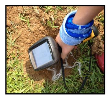
A hand-held XRF device was used to identify and quantify metals contamination at the site, photo by Pan Qingan
