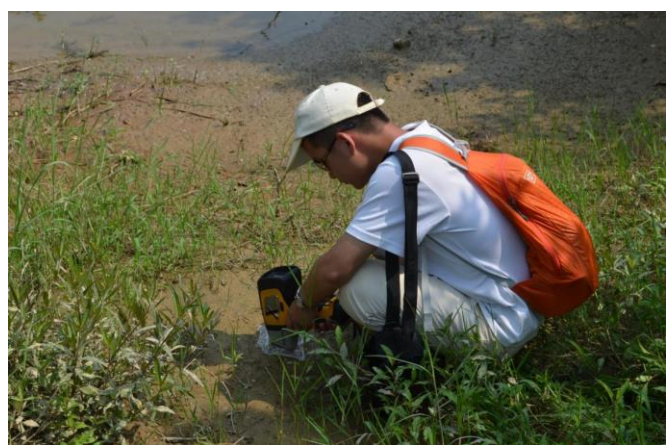
GB staff Pan Qingan is testing the contaminated soil using a hand-held XRF device.
