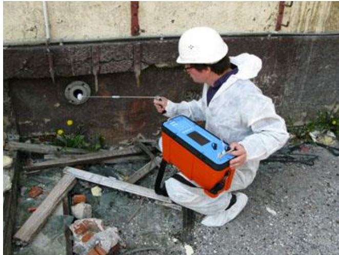
Picture 1: Example of a contaminated site investigator using a portable mercury vapor analyser.
