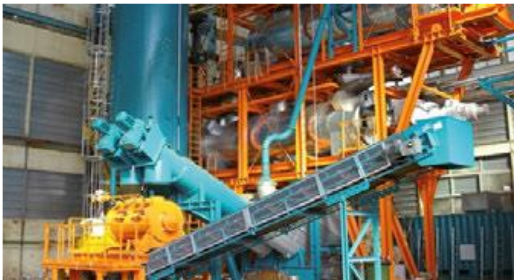
Picture 15. Indirectly heated Vacuum Distillation unit. (Source: econ industries GmbH cited in UNEP/ISWA 2015)
