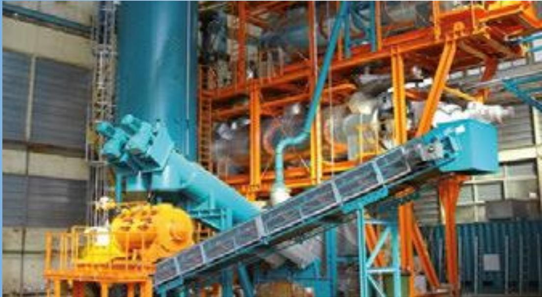
***Indirectly heated vacuum distillation unit.
