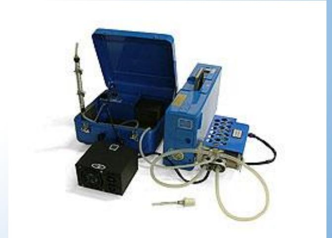
*Ohio Lumex RA915+ Portable Mercury Vapor Analyser, which can also be adapted to sample soil and water.*
