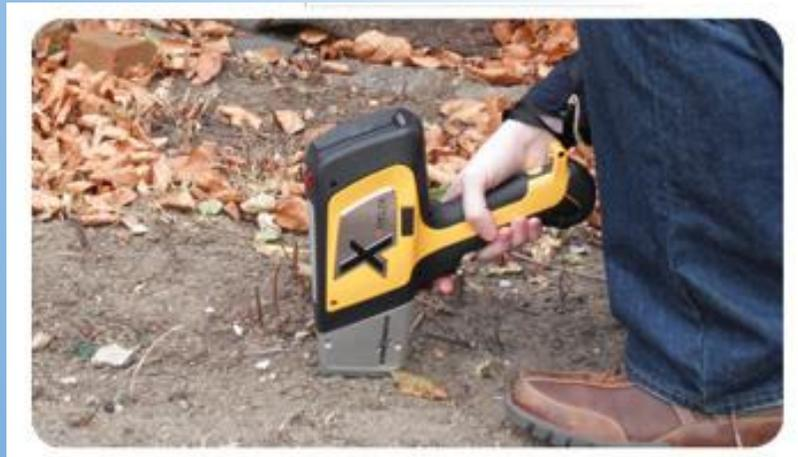
*The Olympus Delta portable X-Ray Fluorescence Analyser*
