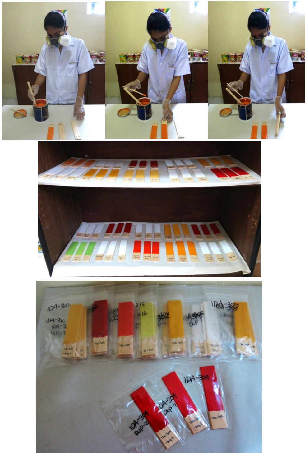
Fig. 8a. Paints stirring and brushing (top). Fig. 8b. Paints samples drying (middle). Fig. 8c. Paints samples packaging (bottom).
