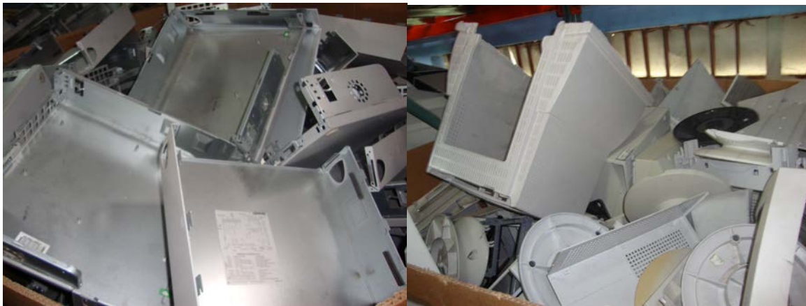
Figure 6: Reusable and recyclable plastic and metal parts of sorted computer components
