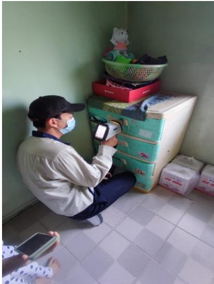
Measuring lead content in toys and environment surroundings the households using a portable X-ray fluorescence device
