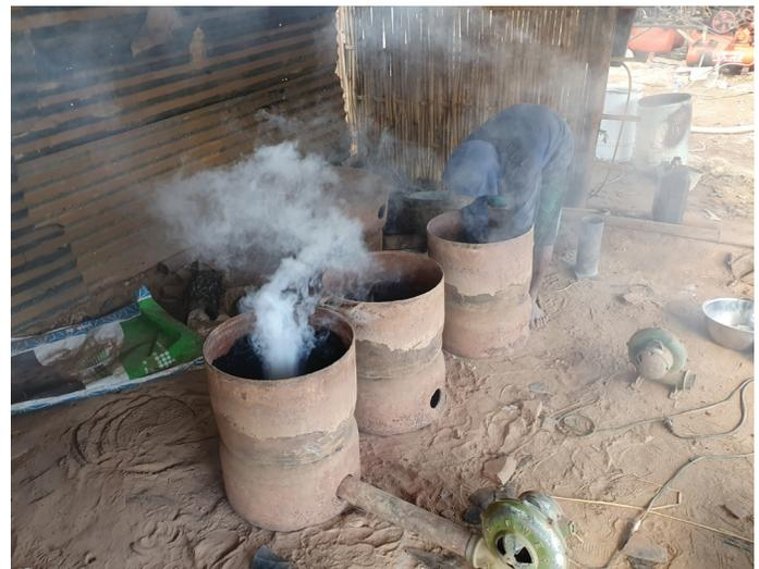
Figure 3. Mercury contaminated cyanidation plant in Indonesia. Tailings stockpiles, liquid releases, emissions from roasted activated carbon laden with gold, mercury and cyanide. Contaminated tailings were given away as construction material. Photos: Lee Bell, IPEN
