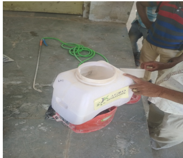
Figure 1 DDT spraying container handled without PPE in an open space
