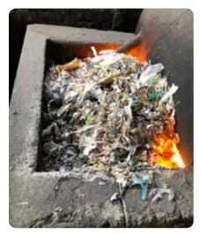
Figure 9. Plastic used as fuel to create steam. Photo: Ecoton
