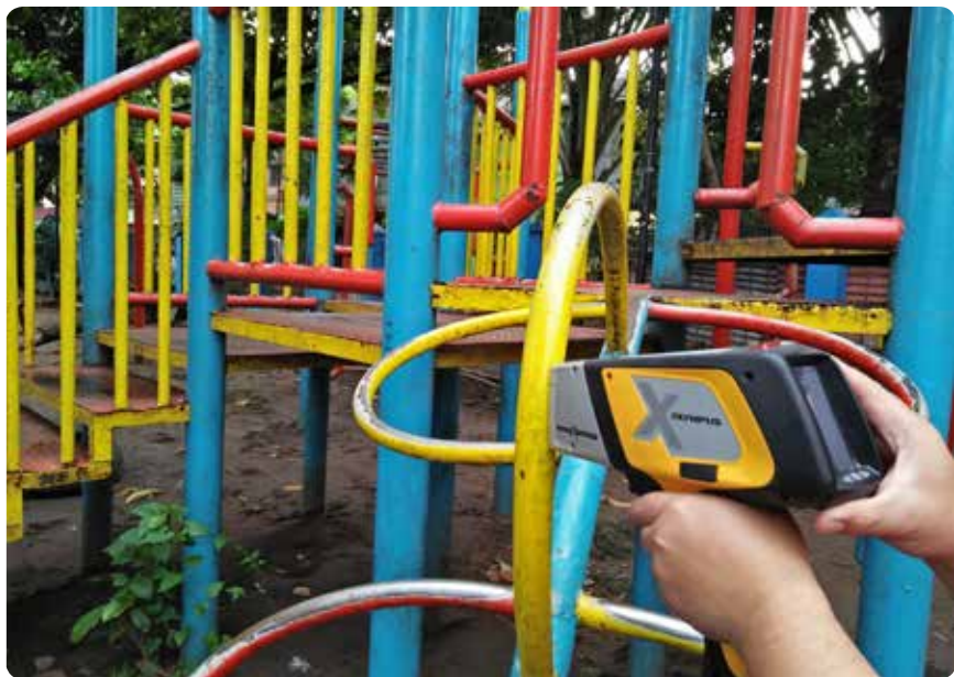
Figure 1. Photo of staff of the EcoWaste Coalition measuring lead content in playground facilities using portable XRF analyzer.
