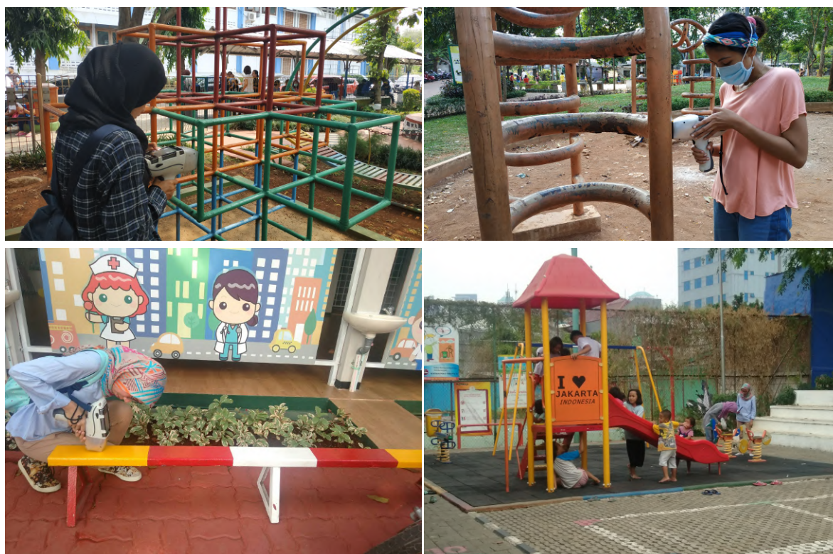
Fig. 13. Many tools in playgrounds around Jakarta used paints with high lead concentration up to 100,000 ppm. Photo credit: Nexus3.
