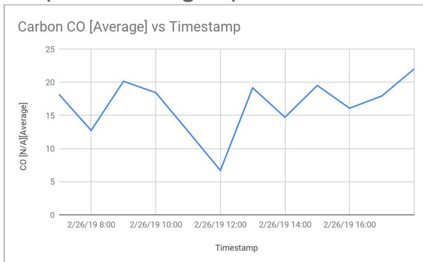
The measured emissions of carbon monoxide during the carbon trial burns were compliant with the EPA licence. No notable peaks could be noticed corresponding to the influence of PFAS injected.
