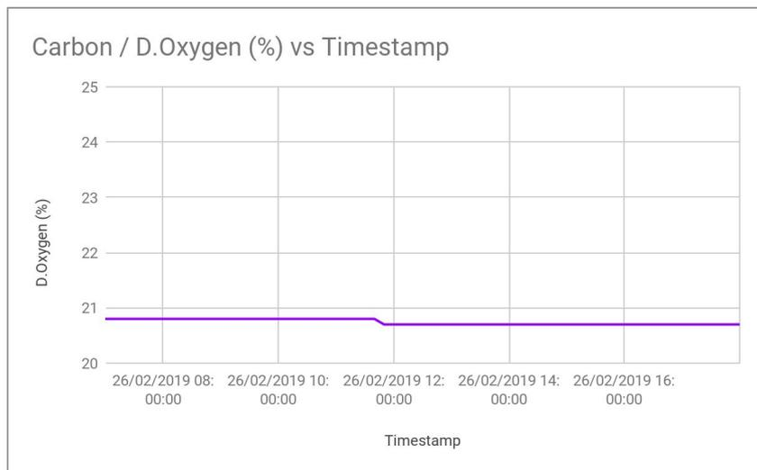
The level of oxygen in the combustion gases were compliant with the 10% minimum limit.
