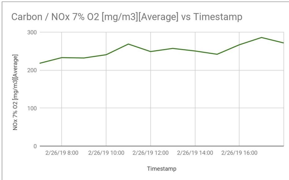
The NOx emissions were compliant with the licence limits during the trial.
