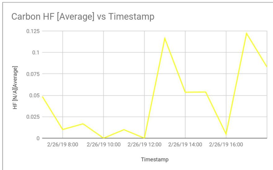
The HF emissions were compliant with the licence limits with two peaks around 13:00 and 17:00 both corresponding to a carbon inhibit message linked to poor loading of chemicals in the scrubbing system.
