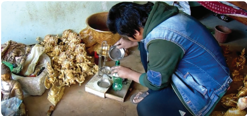
Gold plating worker mixes and burns off mercury-gold amalgam. (CEPHED, Nepal)
