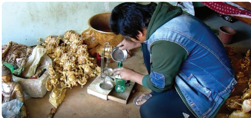
Figure 18. Gold plating worker mixes mercury and gold dust. CEPHED, Nepal
