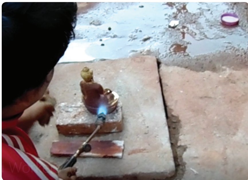
Figure 19. Fire gilder drives off mercury from coating paste to leave gold plate. CEPHED, Nepal
