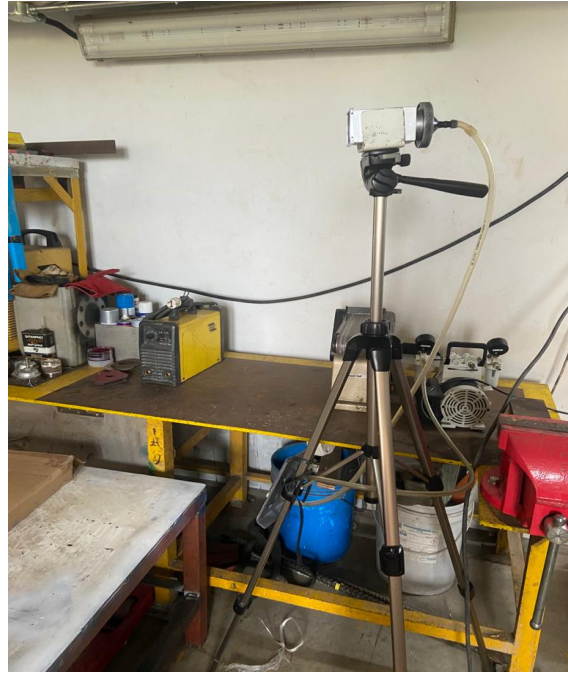
Fig. 15. Low Volume Air Sampler with filter was used to collect samples of lead concentrations indoor air concentrations
