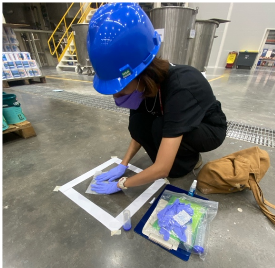
Fig. 16. Lead dust sampling on the floors in some corners of selected rooms.
