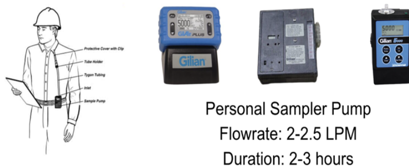
Fig. 11. Personal sampler pump used in this study.
