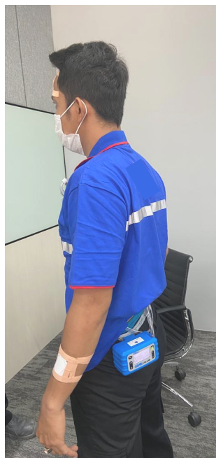
Fig. 12. The personal sampler pump hooked at the back of the waist of a respondent.
