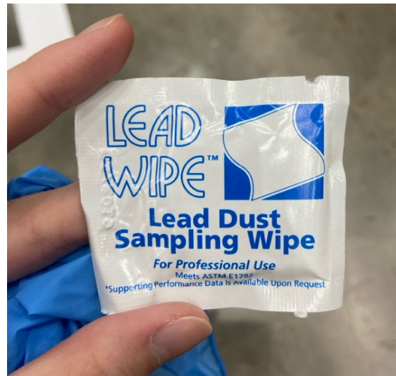
Fig. 17. Lead dust sampling wipe used in this study.
